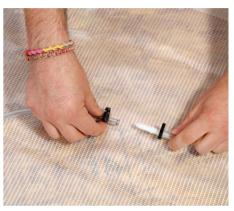
Locate enclosed barbed fitting and 2 hose clamps. Slide one clamp onto the hose and the other clamp onto drain valve that is attached to the diverter. Push the barbed fitting into end of hose and drain valve until secured into place.
