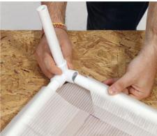
Slide the small support frame through the end pocket. Grasp the corner and insert the end of the support tube into the "Y" connector and snug into place. Repeat on opposite corner. Follow same steps for the other side of diverter.
